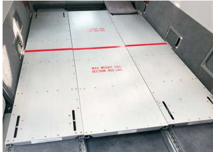
OSA-A installs this shelf cargo floor in all of its C-12 detachments throughout the world. It allows an increase in light cargo carrying abilities, ensures that all cargo is safely secured and keeps the weight properly distributed throughout the aircraft cabin.
