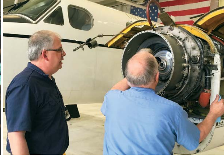
DynCorp International contractors handle all maintenance for the OSA-A fleet of Beechcraft King Air C-12 aircraft. Here, DynCorp's Aaron DeMoss (left) and Doug Kratz (right) conduct a hot section inspection on a C-12U.
