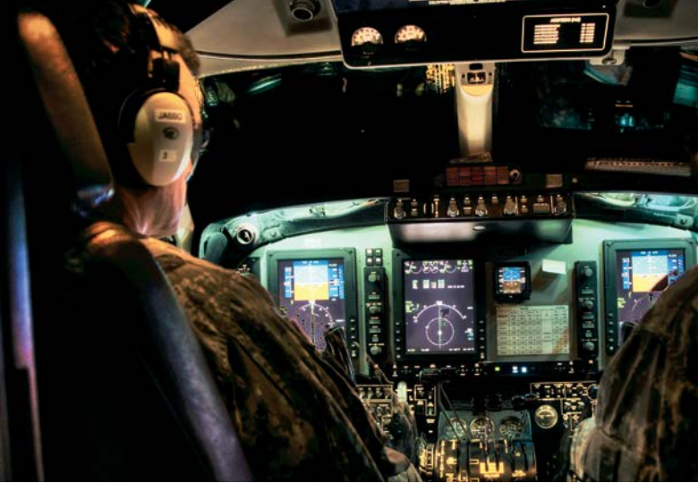
The Army National Guard has five C-12Vs that have the Rockwell Collins Pro Line 21 avionics suite, while a majority of the C-12s have the company's FMS-3000 system.
