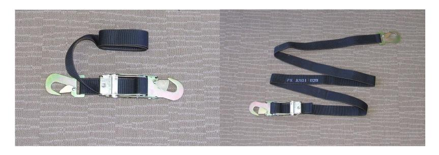
Cargo Strap AM01 120 minimum length is 15 inches and maximum is 104 inches. The AM01 120 Cargo Strap is rated for over 3,200 pounds static and can secure 175 pounds of freight per strap at an 18 g loading.
