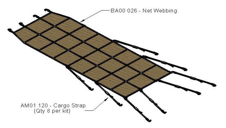
Cargo Net Assembly FA00 003 is comprised of the following parts:
