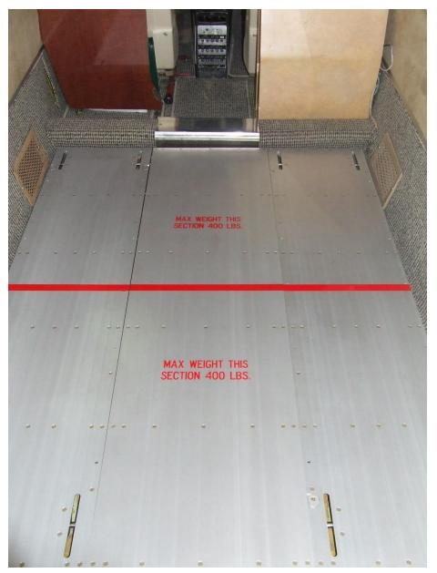
The King Air 90 series cargo configuration is shown to the left. This configuration will allow for up to 800 pounds of freight in the cabin.
