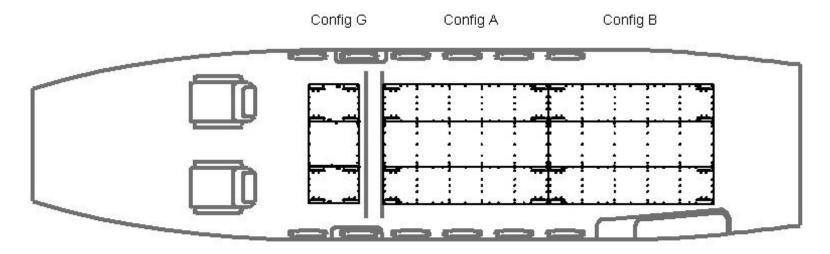
Aerospace Resources King Air 350 **Configuration G** has a weight capacity of 300 pounds of freight and is 20.0 inches by 46.8 inches. The three decks used for Config G are contained in **Kit K004** (see Kits, Assemblies and Parts). Recommended for use with **Cargo Net Assembly FA00 003**.
