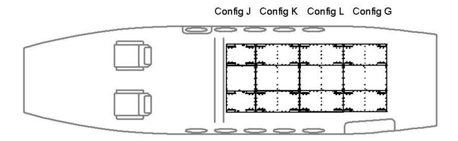
Aerospace Resources King Air 200 and 250 **Configuration J** has a weight capacity of 300 pounds of freight and is 20.0 inches by 46.8 inches. The three decks used for Config J are contained in **Kit K004** (see Kits, Assemblies and Parts). Recommended for use with **Cargo Net Assembly FA00 003**.
