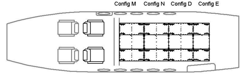
Aerospace Resources King Air 200 and 250 **Configurations M, N and D** have a weight capacity of 400 pounds of freight and is 30.0 inches by 46.8 inches. The three decks used for Config M, N and D are contained in **Kit K003** (see Kits, Assemblies and Parts). Recommended for use with **Cargo Net Assembly FA00 003**. Also, **Restraint Bar FA00 005** may be used at operator's discretion to keep small, heavy cargo from shifting longitudinally under the Cargo Net Assembly.
