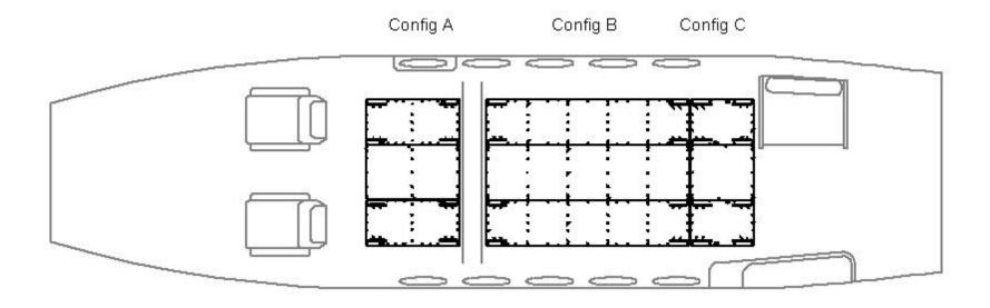
Aerospace Resources King Air 200 and 250 **Configuration A** has a weight capacity of 400 pounds of freight and is 30.0 inches by 46.8 inches. The three decks used for Config A are contained in **Kit K003** (see Kits, Assemblies and Parts). Recommended for use with **Cargo Net Assembly FA00 003**. Also, **Restraint Bar FA00 005** may be used at operator's discretion to keep cargo from shifting longitudinally under the Cargo Net Assembly.
