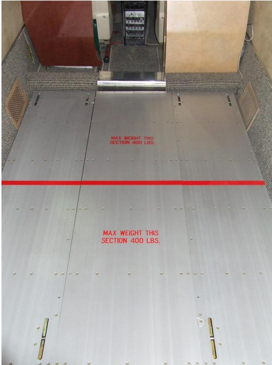
The King Air 90 series cargo configuration is shown to the right. This configuration will allow for up to 800 pounds of freight in the cabin.
